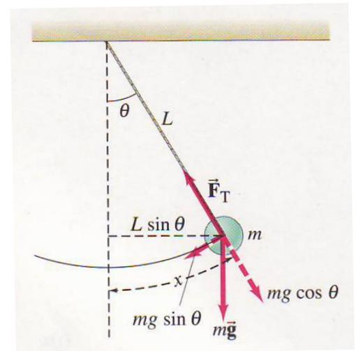
**Figure 3:** A simple pendulum. (From Douglas C. Giancoli, *Physics: Principles with Applications*, 6<sup>th</sup> edition, Ch. 11, Pearson Prentice Hall, 2005)
