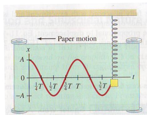
**Figure 2:** Displacement of a SHO as a function of time. (From Douglas C. Giancoli, *Physics: Principles with Applications*, 6<sup>th</sup> edition, Ch. 11, Pearson Prentice Hall, 2005)
